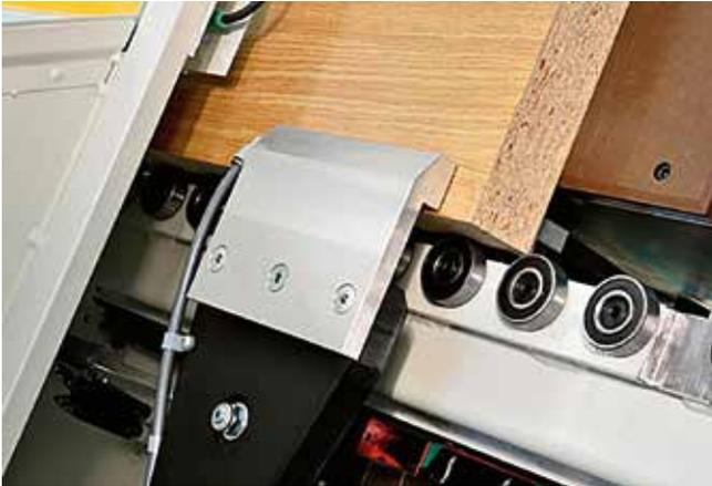
**Maximum piece stability and high machining quality**, with the mobile clamp with floating opening that does not require any adjustment and the Bakelite non-scratch table that guarantees high machining quality also for panels with delicate surfaces.
