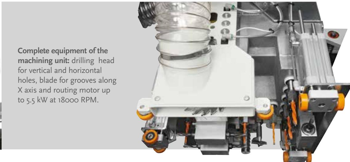
**Complete equipment of the machining unit:** drilling head for vertical and horizontal holes, blade for grooves along X axis and routing motor up to 5,5 kW at 18000 RPM.
