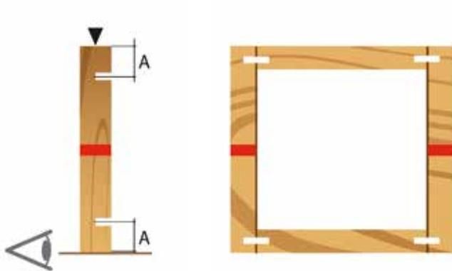
**Perfect joints,** with the automatic reading of the piece length. Any difference between the actual length of the panel and the length set is detected by the highly precise laser reader to ensure **perfect alignment**.
