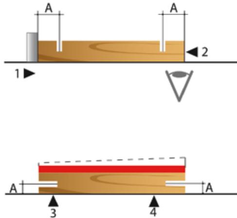
**Perfect finish**, drilling on the top side allows external part of the panel to be referenced, hiding any squaring defects of the piece.
