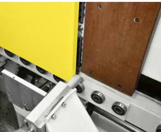
**Highly versatile**, the programmable side reference stop lets you machine pieces with dowels already inserted or with routing already carried out.
